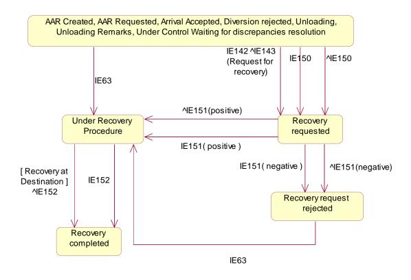
Figure 75: State Transition Diagram of the recovery states in the Destination in the NCTS Phase 4
