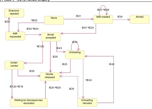
Figure 74: State Transition Diagram for Office of Destination in NCTS Phase 4 without Recovery States
