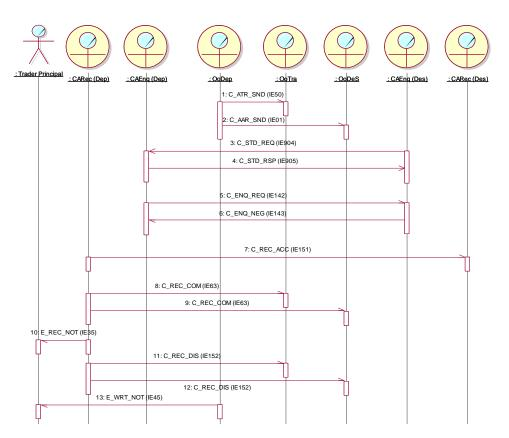
Figure 64: Recovery at Departure – Destination's Recovery Request rejected
